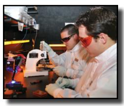
This team is testing resin curing lights to determine their ability to cure a variety of resin-based composites.
