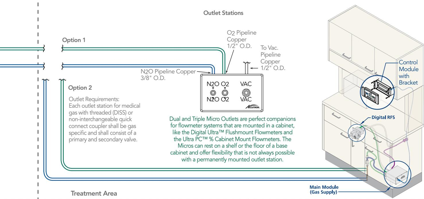
**Medical Gas systems must be installed by a licensed medical gas installer (i.e. ASSE 6010) and be verified by a licensed medical gas verifier (i.e. ASSE 6030) and must be installed in compliance with NFPA 99 requirements.**
