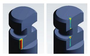
Previous Generation: High loads on the edge of the tool could result in significant deformation. This results in shaft interference in the clamping system.
